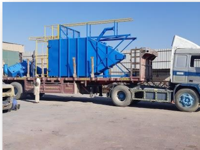
Bag Filter – Cement Factory
